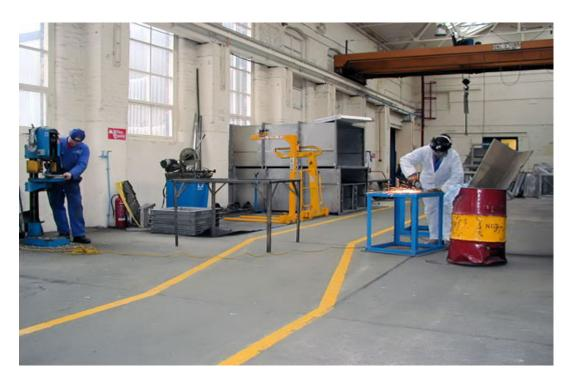
Okay, how many hazards did you spot in the photo? Here are several: tripping hazard (cord), no gloves on worker (left), fire extinguisher obstructed, poor housekeeping (teetering box on top of bins) and fire hazard (grinding near flammables in refuse can).
